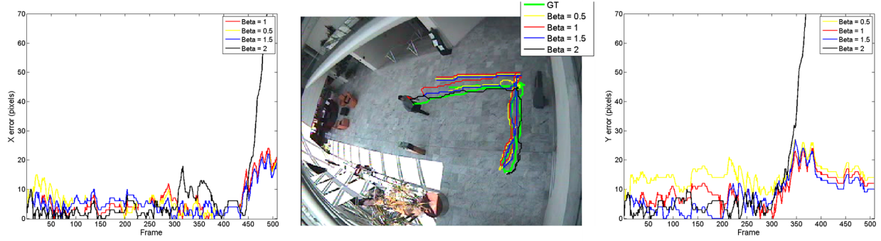
Figure 3: Centre image: Trajectories of the F-score tracker when varying \beta . Yellow: \beta = 0.5 , red: \beta = 1 , blue: \beta = 1.5 , black: \beta = 2 . Left image: error in pixels on the X coordinate compared with the ground truth. Right: error (in pixels) on the Y coordinate.
